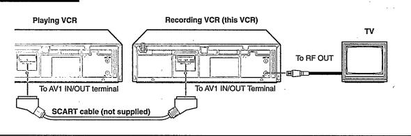
Dubbing from any VHS VCR (or video camera) to another is simple. Explanations on this page uses this VCR as the recording VCR. Refer also to the manual supplied with the other VCR (for playback).
